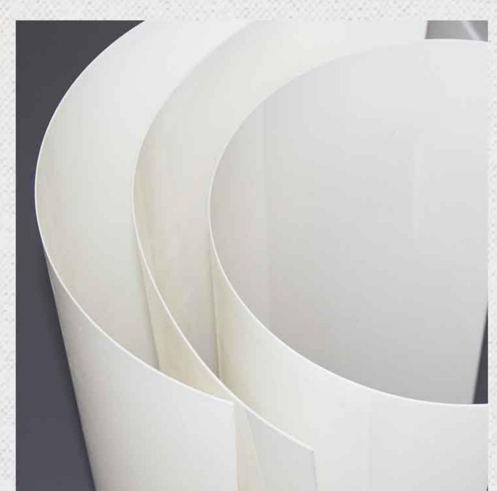
NMN 6640 P-PAa/F-PET/P-PAa This product is a kind of three- layer composite material with NOMEX paper adhered to both sides of polyester film. It has excellent heat resistance and tear resistance by its paper and good dielectric strength and mechanical strength by its film. The product is used as insulation material for F/H class electric machines.
